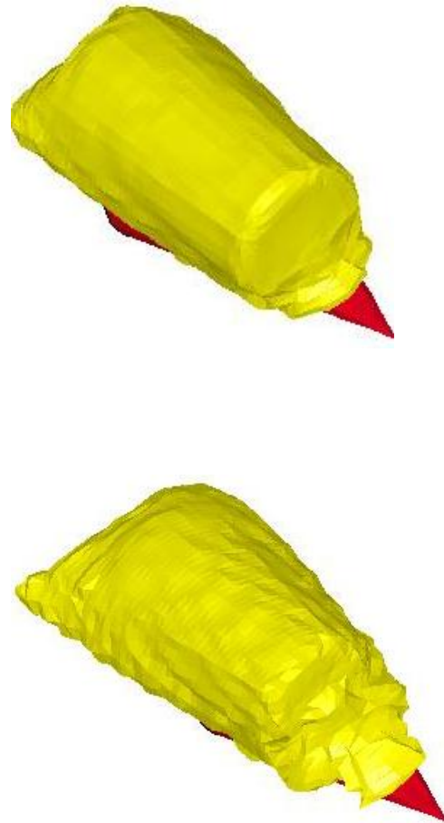
Fig 2: flow pattern of bird on cone
